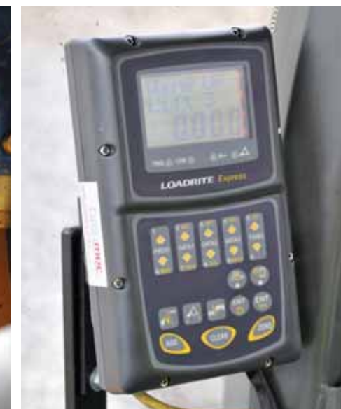
A rotary trigger monitors the angle of the arms and transducers measure the hydraulic pressure, the data being available in a number of media including the control screen.
