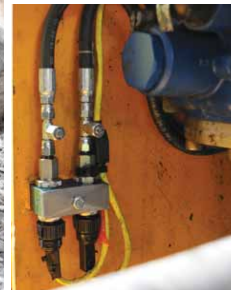
A rotary trigger monitors the angle of the arms and transducers measure the hydraulic pressure, the data being available in a number of media including the control screen.
