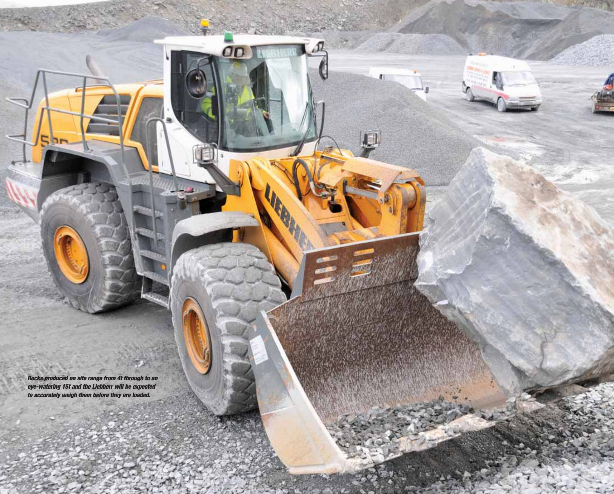
A rotary trigger monitors the angle of the arms and transducers measure the hydraulic pressure, the data being available in a number of media including the control screen.
